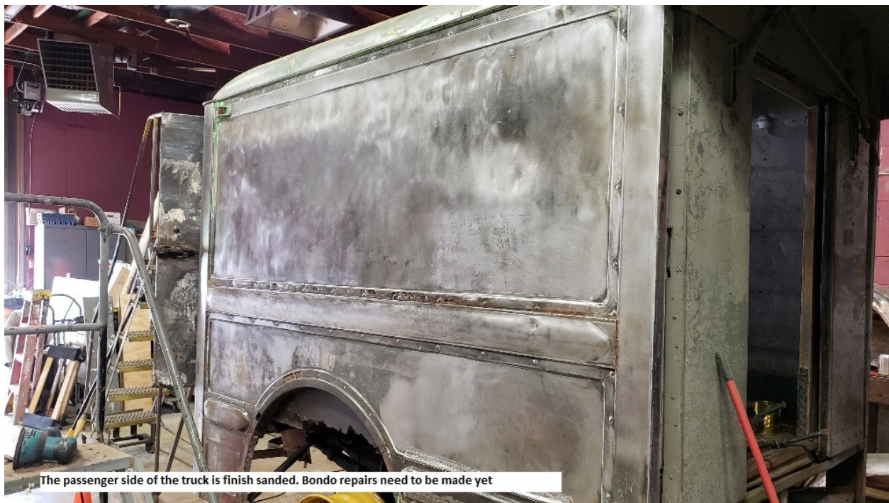
The passenger side of the truck is finish sanded. Bondo repairs need to be made yet
