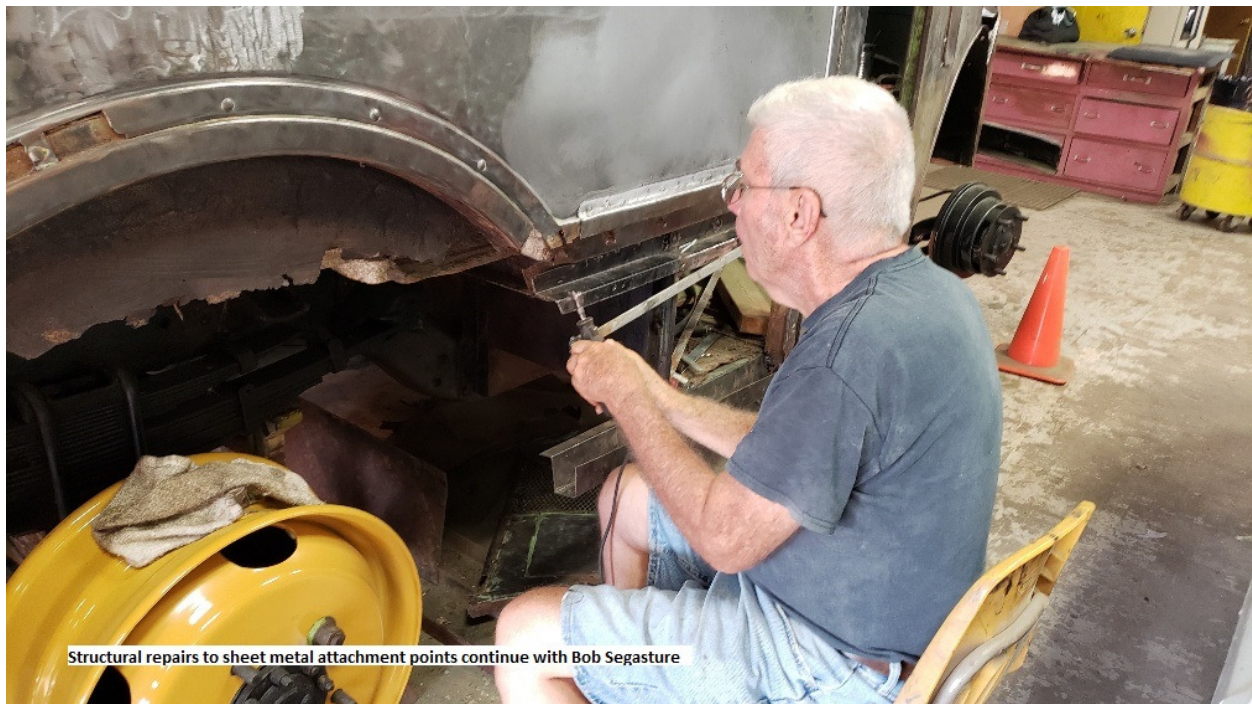
Structural repairs to sheet metal attachment points continue with Bob Segasture
