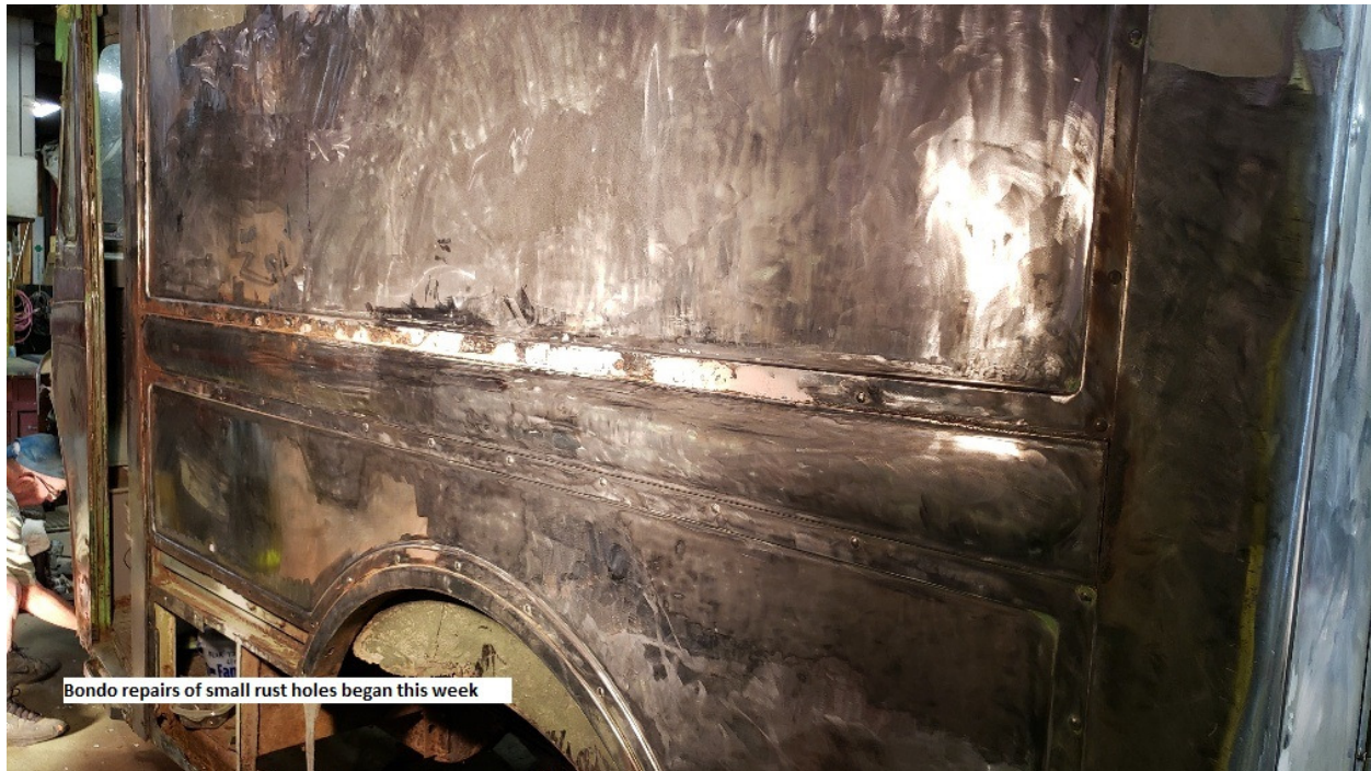
Bondo repairs of small rust holes began this week
